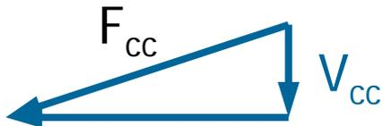
$$V_{Rd,ST} = V_{Rd,s} + V_{cc} + V_P \geq V_{Ed} \quad \checkmark$$
